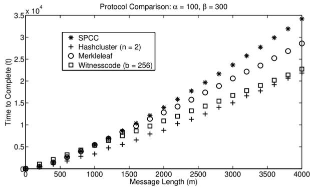
Figure 10: The expected time  $t$  to complete a message exchange for all four protocols, with  $\alpha = 100$  and  $\beta = 300$ . The SPCC and Merkleleaf schemes behave similarly for  $m < 1500$ , after which they diverge due to the coding gain in the Merkleleaf scheme.
