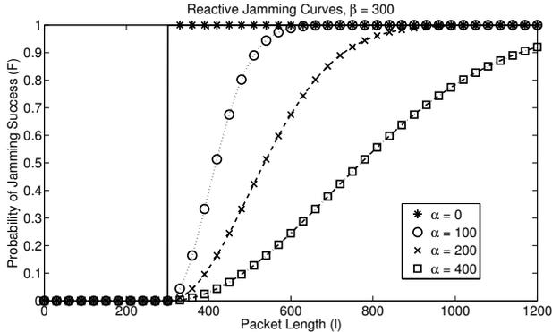
Figure 2: Reactive jamming distributions for various Rayleigh parameter choices, which maps the length of a packet to its probability of being reactively jammed, with  $\beta = 300$  and  $\alpha \in \{0, 100, 200, 400\}$ .
