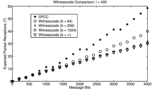
Figure 6: The average number of packet receptions for the Witnesscode scheme is evaluated for various coding values  $b$ , with the SPCC scheme included for reference. The case of  $b = \infty$  represents the optimal coding case with infinite computational overhead.
