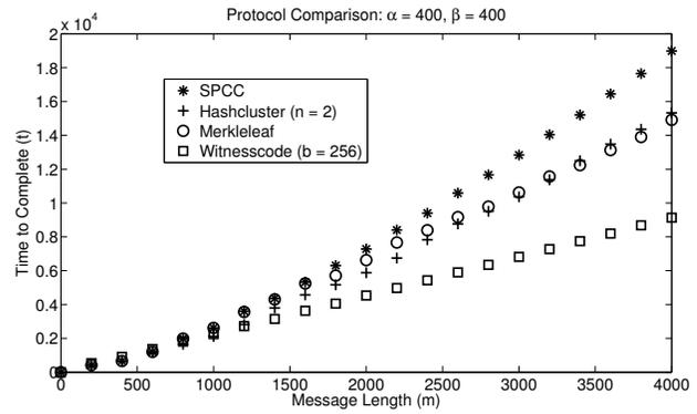
Figure 11: The expected time  $t$  to complete a message exchange for all four protocols, with  $\alpha = 400$  and  $\beta = 400$ . The Witnesscode greatly outperforms the other protocols for  $m > 1200$ , due to a large coding gain, and the Merkleleaf and Hashcluster schemes perform similarly for all  $m$ .
