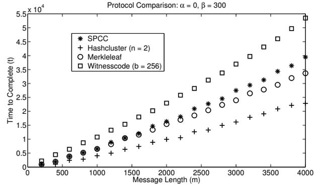
Figure 9: The expected time  $t$  to complete a message exchange for all four protocols, with  $\alpha = 0$  and  $\beta = 300$ . The Witnesscode scheme does significantly worse than the other schemes and Hashcluster does significantly better, due to their respective fraction of data spent on verification.
