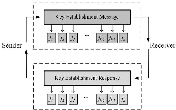
Figure 1: The logical exchange of key establishment messages between the sender and receiver requires only two message exchanges. Each message is disassembled into a collection of  $k$  fragments  $f_i$ .
