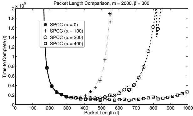
Figure 7: Tradeoff between fragment verification and reactive jamming resilience, mapping packet length  $l$  to message exchange time  $t$ , with  $m = 2000$ ,  $\beta = 300$ , and  $\alpha \in \{0, 100, 200, 400\}$ .
