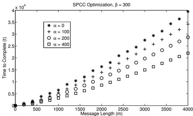
Figure 8: Time  $t$  to complete the message exchange after performing packet length optimization on the SPCC scheme.  $\alpha$  is varied among 0, 100, 200, 400 and  $\beta = 300$ . The  $\alpha = 0$  case represents the performance baseline of the optimization.
